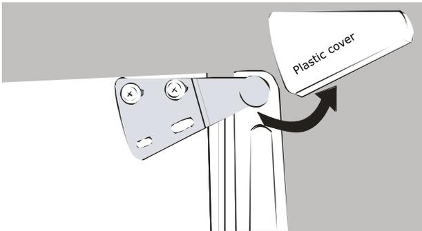
4. To install the bracket on the left side of the appliance, screw the two screws through the bracket and into the top of the appliance. Slide the door back on to the top hinge. Ensure the door is face up. Replace the plastic cover on the top bracket by pressing down until it clicks into position.
