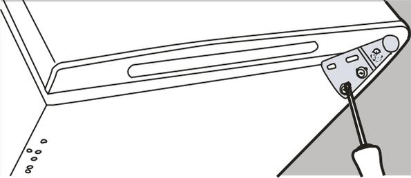
5. Screw the bottom hinge into place on the new side. Replace the foot on the other side.
