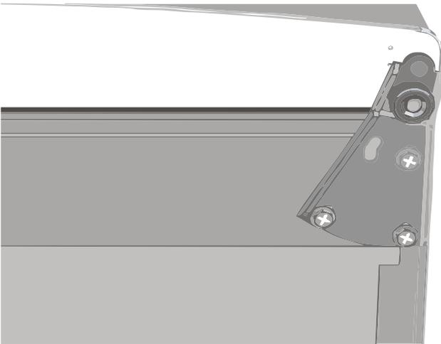
6. Check that the door is aligned horizontally and vertically and that the seals are closed on all sides before finally tightening the bottom hinge. Re-adjust the leveling feet.
