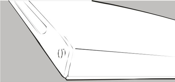
3. Remove the plastic cover from door hinge first. Then unscrew the two screws from top bracket and replace on the other side.
