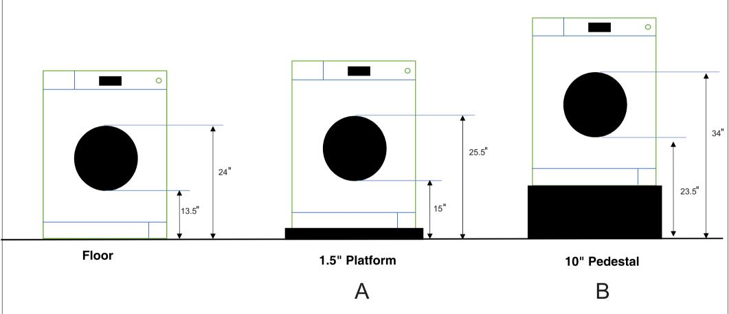
For Super Combo Washer-Dryer, bottom of the opening of the laundry compartment is located at 13.5 inches. Hence Super Combo Washer-Dryer cannot comply with ADA standards. It can only comply with ADA if either of the conditions (A or B) are complied with.
